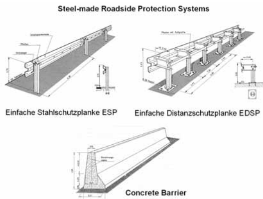
Figure 1. Two steel-guard rails and a concrete barrier common for German roads and investigated with full-scale crash tests
